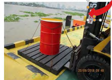
Tied equipment by ropes prior moved from the jetty front by forklift, then carried to storage area by pick-up truck
